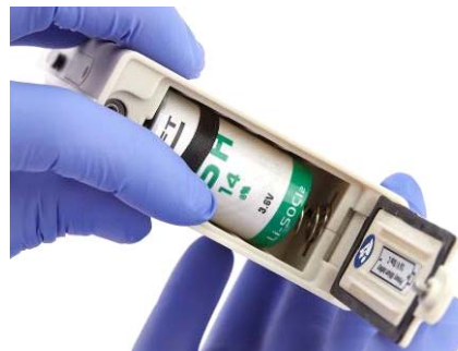
Figure 10: Close the battery compartment cover with the tool by securing the battery compartment screw. Do not jam the battery removal strip.
