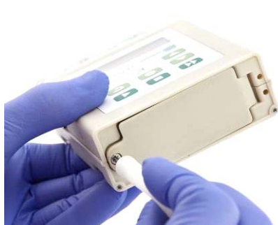
Figure 8: Open the battery compartment with the provided tool.
