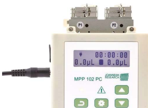
Figure 11: Alternative operation of the pump via power supply.
